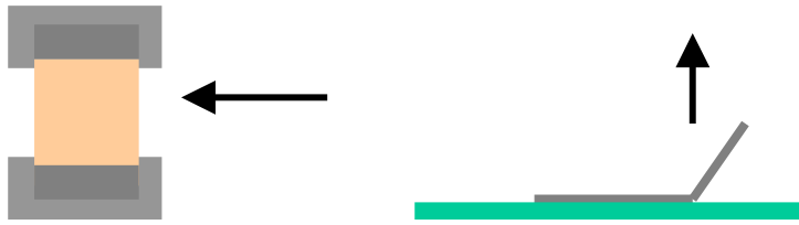
Schematic diagram indicating force application to SMD components
