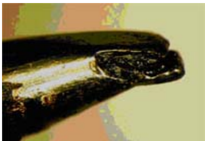
Lead-free tip failure after 3 weeks
