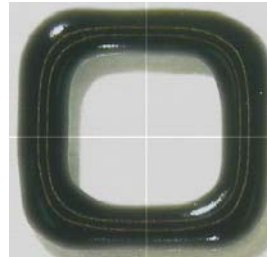
Figure 6. Cavity wall formed by jetting silicone adhesive
